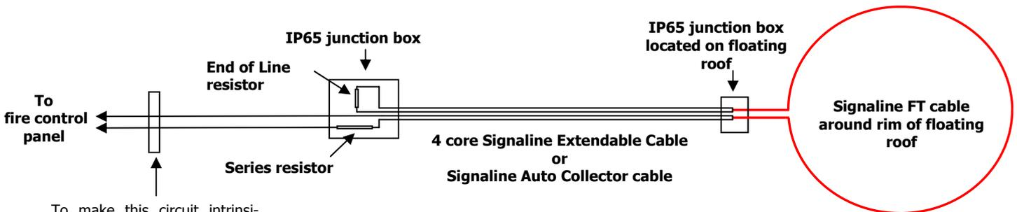
To make this circuit intrinsically safe (EEx ia), a suitable IS barrier such as the MTL5061 is placed in the circuit as per diagram. The barrier MUST be located in the safe area of the site.
