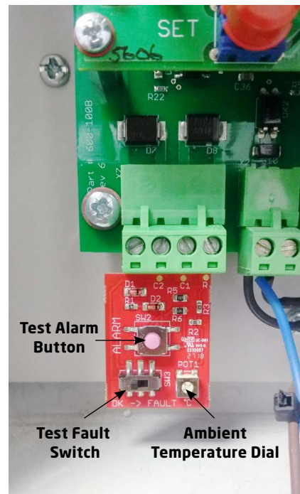
Figure 12: Analogue test board installed in control unit
