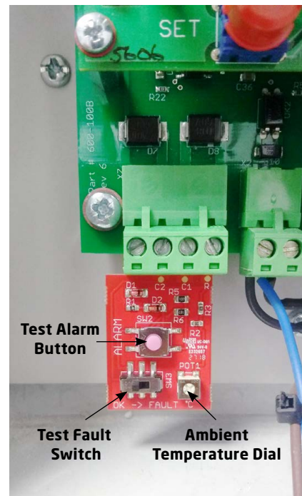
Figure 12: Analogue test board installed in control unit
