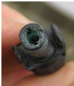
Example of an unprotected connector that has been contaminated (Picture/Illustration of Stäubli, Switzerland)
